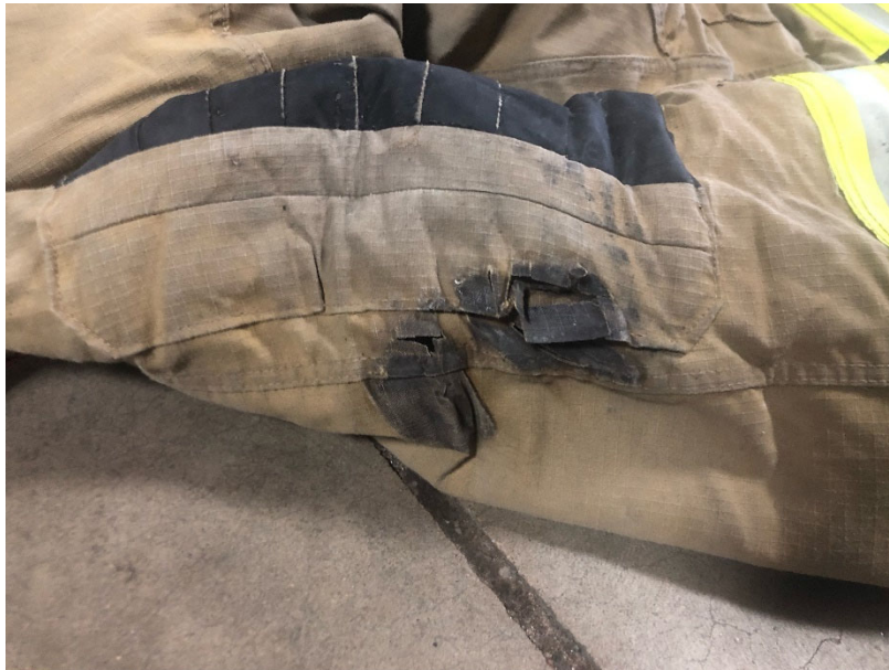
Above: A pair of bunker pants were burned through during fire suppression)
