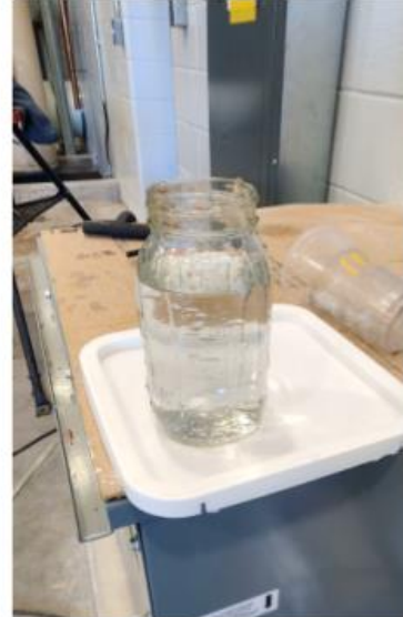
Structure 120 (PFAS Treatment Building), set of photos showing fines at the start of a GAC backwashing sequence, the middle and the end with fines washed out.
