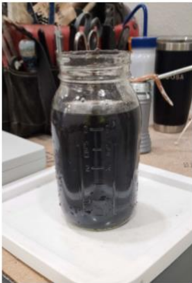
Structure 120 (PFAS Treatment Building), set of photos showing fines at the start of a GAC backwashing sequence, the middle and the end with fines washed out.
