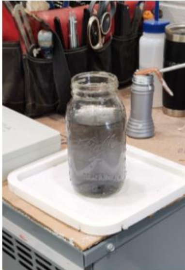
Structure 120 (PFAS Treatment Building), set of photos showing fines at the start of a GAC backwashing sequence, the middle and the end with fines washed out.
