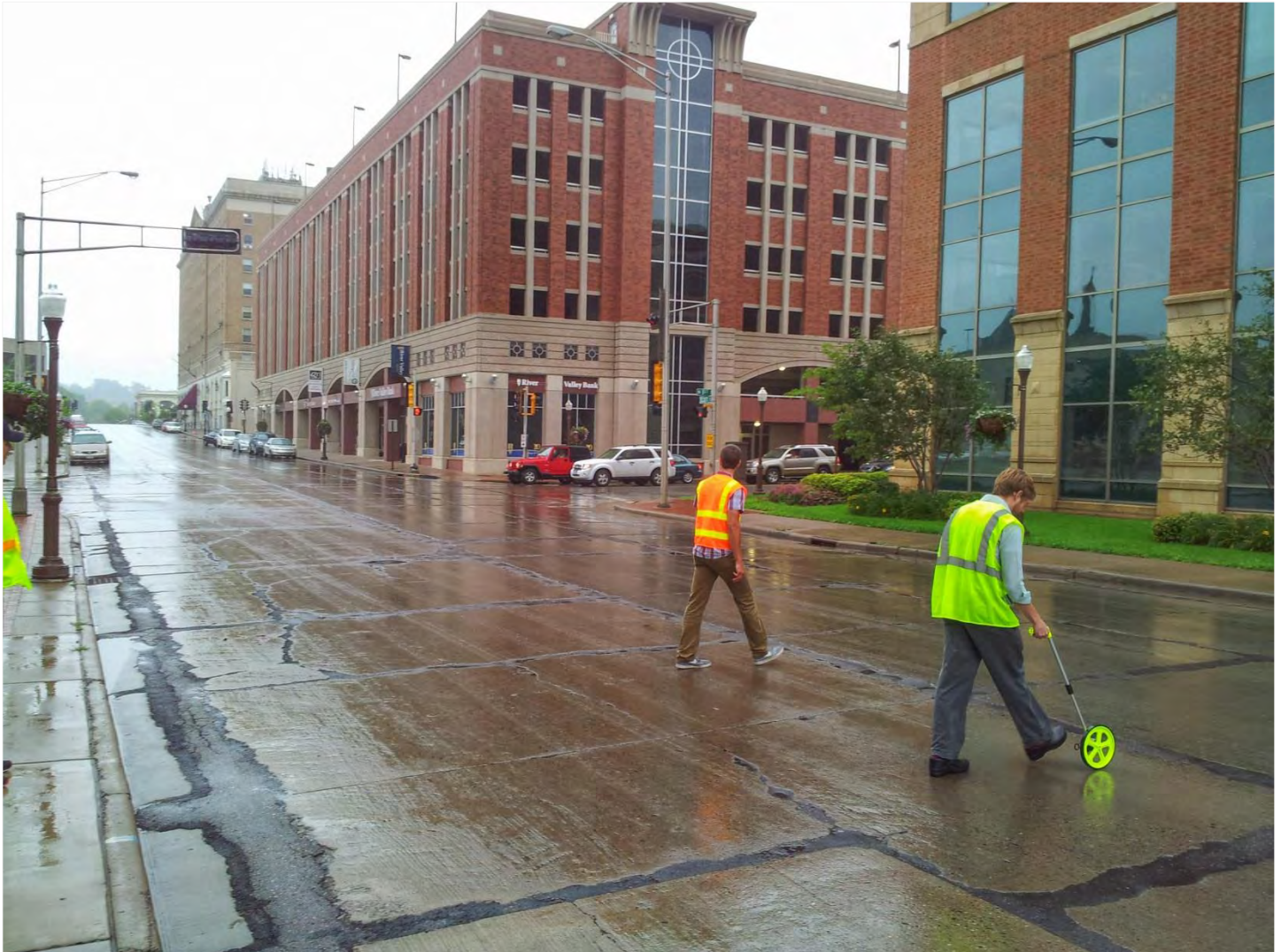
Members of the planning team measuring street width as part of its field work performed in September 2014.
